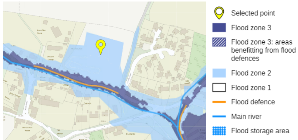
Figure 1: Extract from Environmental Agency showing Flood Zones.
